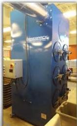
After research was conducted on the capacity required to effectively capture the dust, it was agreed that the A.C.T. LaserPack 6 was the best option for this application. It is designed for use in fiber laser applications and is equipped with an integrated spark trap, pre-wired controls, noise attenuation blower enclosure, and features a remote start feature so the dust collector can be controlled from the fiber laser machine.
